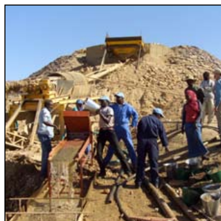
Team of trainers running sluices.
