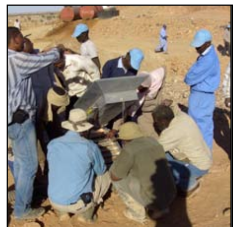
Imported dry sluice tested out.
