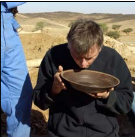
Tapping and blowing technique requires no mercury and is appropriate when yield is small.
