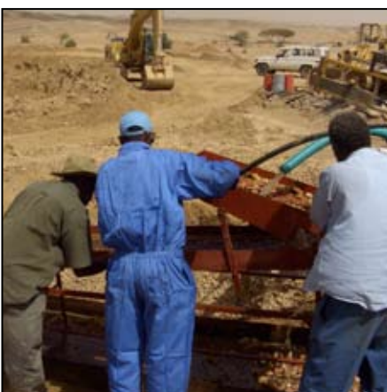
Setting up locally made sluices in the field for testing.
